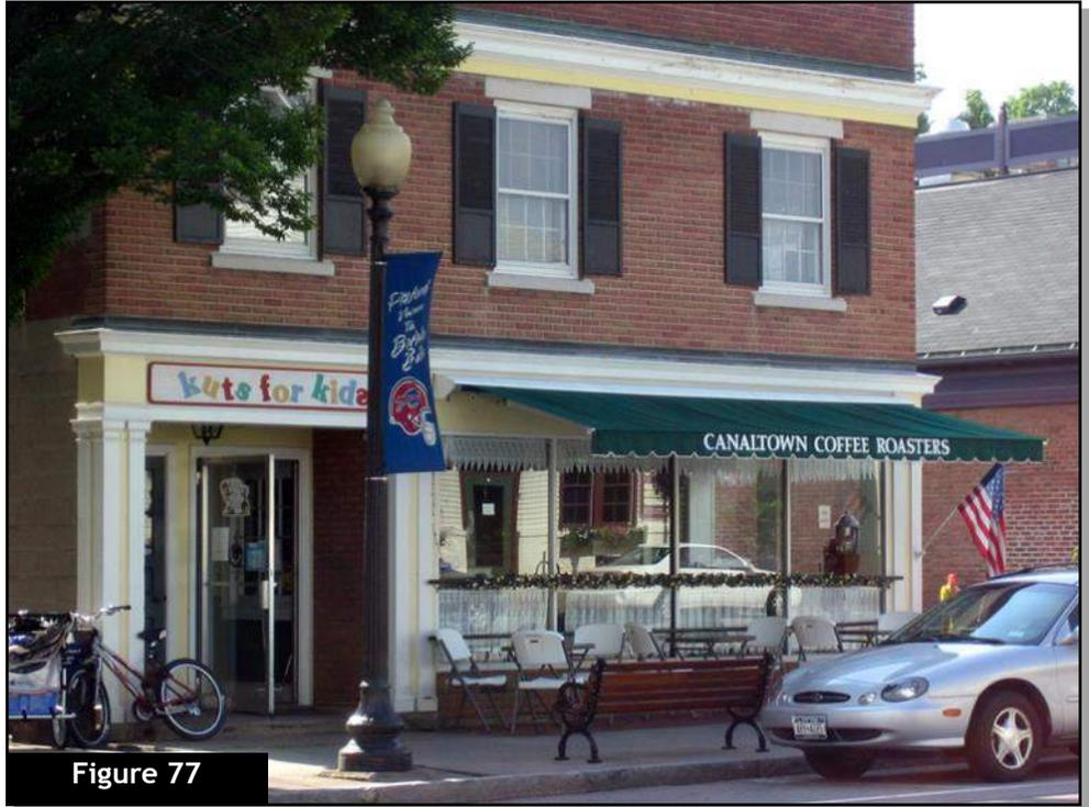
*Awnings are a high quality design element that define the purpose and volume of outdoor spaces. They also add visual variety and distinction to building façade components [§ 112-17G(4)(h)]. The building in Figure 77 also displays a significant amount of transparency and the successful use of a cornice to differentiate the 1st floor from upper stories.*
