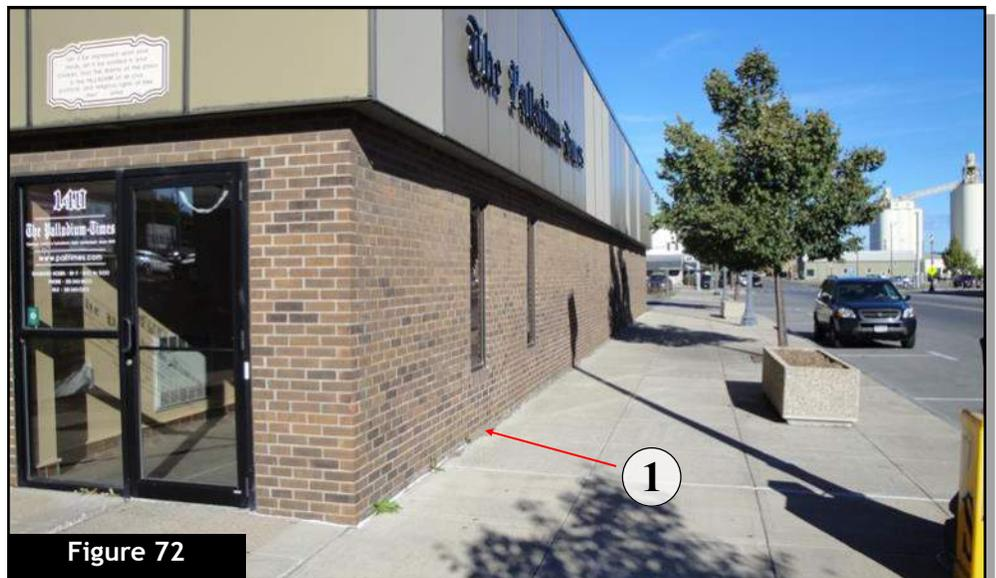
*The building façade shall not abruptly end at the sidewalk (1). The building shall have a base of material that anchors the structure to the site [§ 112-17G(2)(a)]*
